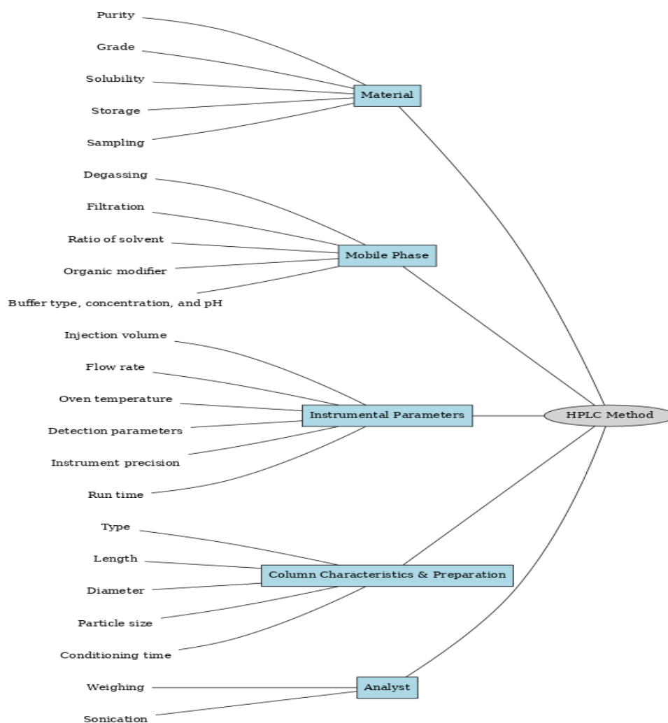
Figure 2: The Ishikawa (also called the fishbone) chart to find potential parameters in HPLC method Development
